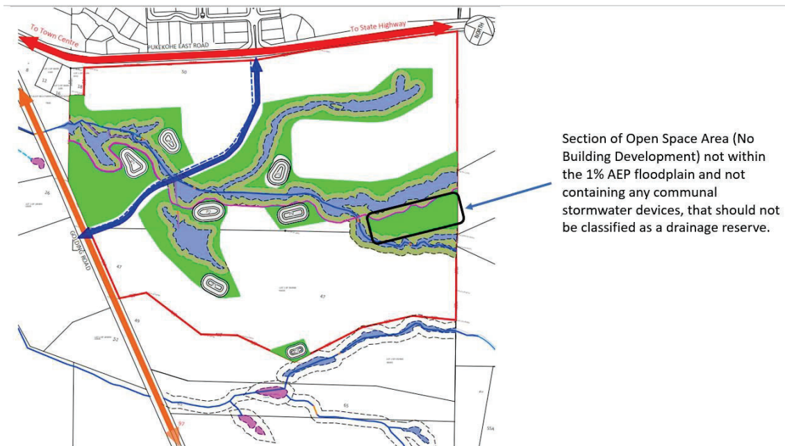
Figure 1. The area of Open Space Area (No Building Development) that lies between the two streams at the eastern extent of the plan change area (outlined in black) should not be drainage reserve as this area is not within the 1% AEP floodplain and no communal stormwater ponds are located in this area.
